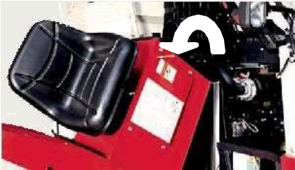
Tilting seat arrangement for easy Engine maintenance
