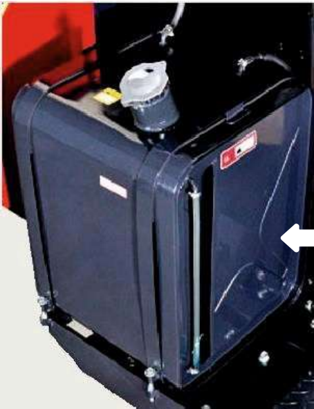
Large-capacity fuel tank (90 L) with fuel indicator
