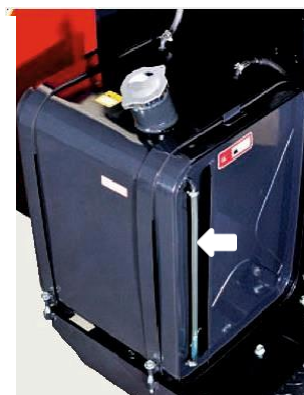
Large-capacity fuel tank (90 L) with fuel indicator
