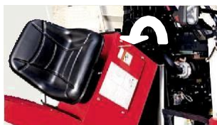
Tilting seat arrangement for easy Engine maintenance
